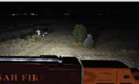
PERIMETER LIGHTS 1 WHELEN M9 AND 2 FIRETECH FT-B-45 (46" LED STICKS) ON EACH SIDE OF THE TRUCK
