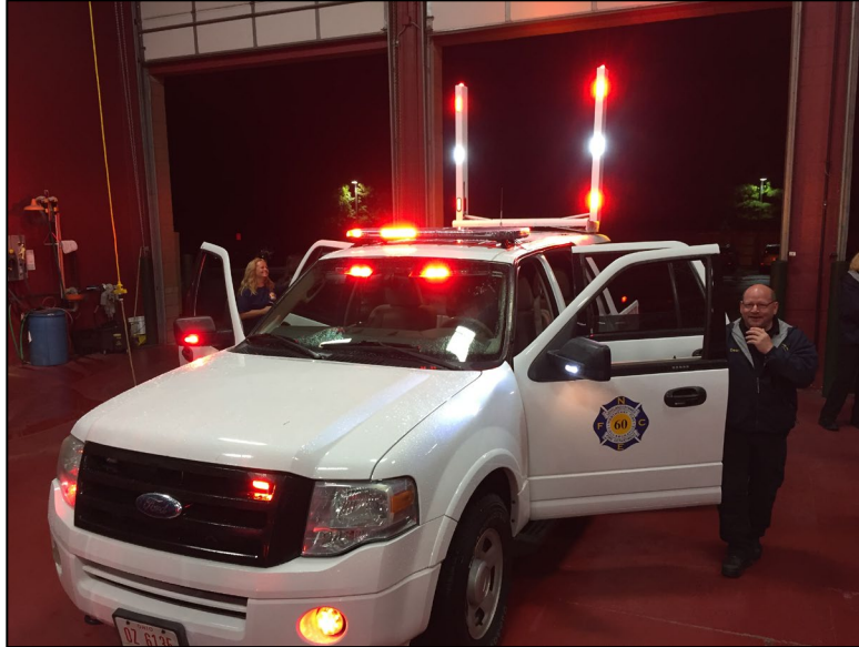
Figure 11: Another example of a high-rise light bar, this one on a vehicle from the Loveland-Symmes Fire Department. Photo credit: Loveland-Symmes Fire Department.
