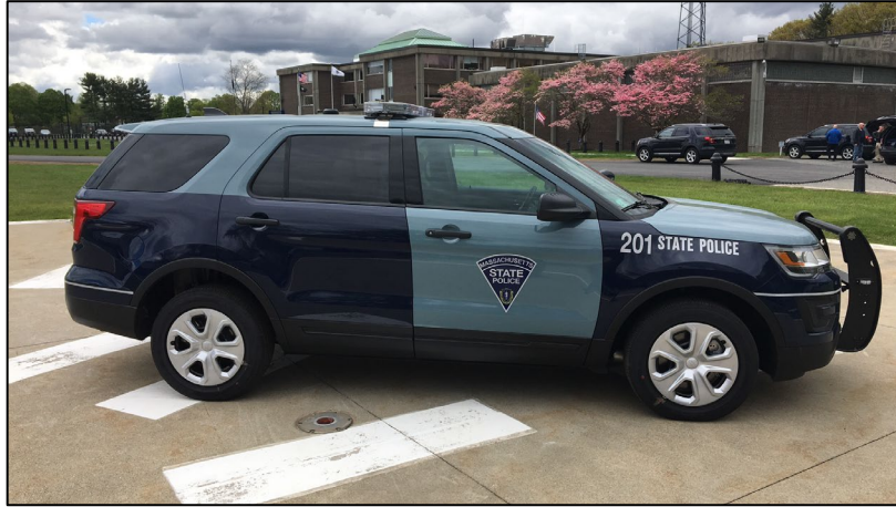
Figure 6: Side markings of MSP vehicles are retroreflective. Photo credit: Massachusetts State Police.
