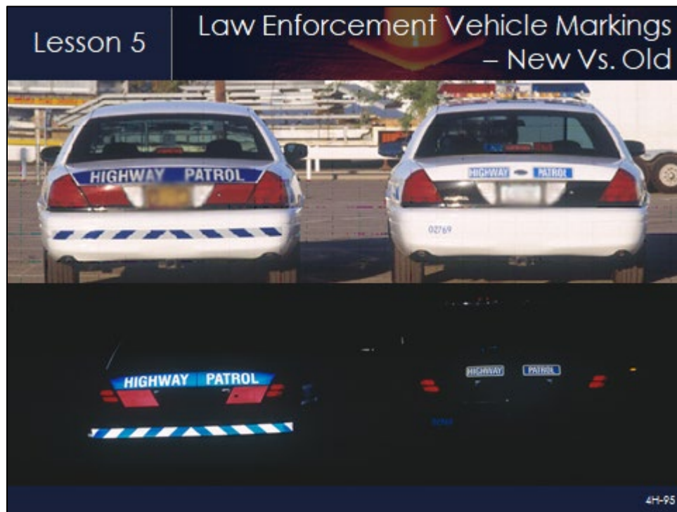
Figure 1. Comparison of conspicuity of "new" vs. "old" retroreflective vehicle markings on the rear of Arizona Highway Patrol cruisers. Image from the National TIM Training Program (Rev 7/13). Photo Credit: Federal Highway Administration.
