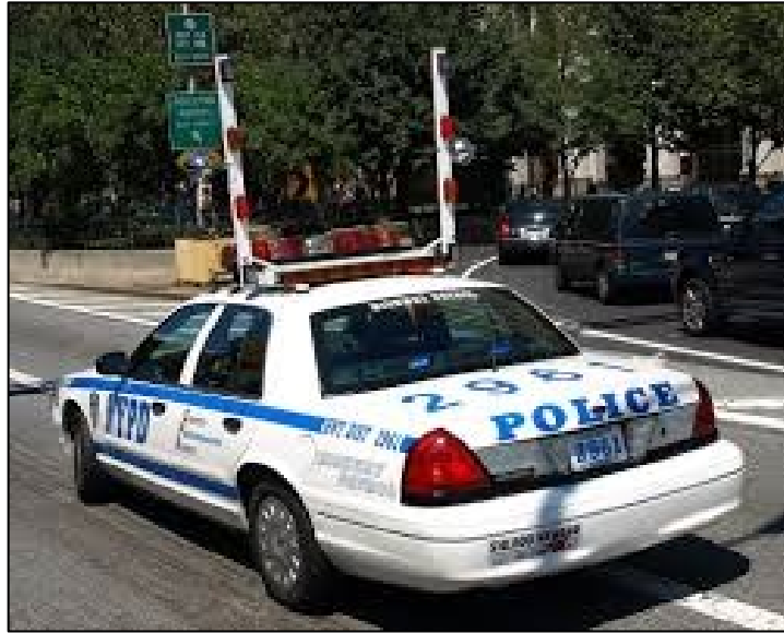
Figure 10: Multi-level or high-rise lighting system in deployed mode. Photo credit: Richard Pepe, NYPD Retired.
