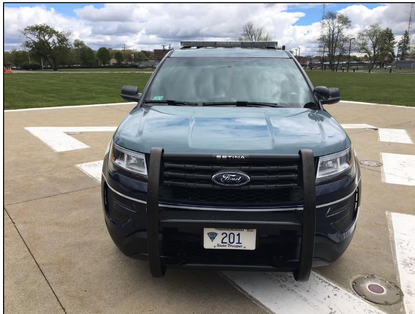
Figure 7: Thin strip of retroreflective material is visible above the front bumper of this MSP vehicle. Photo credit: Massachusetts State Police.
