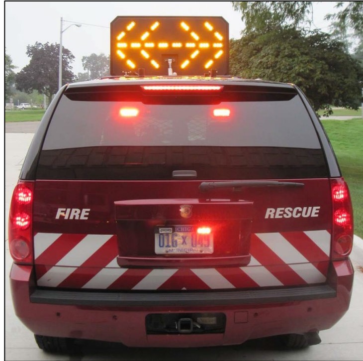
Figure 19: Livonia (MI) Fire & Rescue vehicle outfitted with a high-mounted arrow board for traffic control. Photo credit: Livonia (MI) Fire & Rescue.
