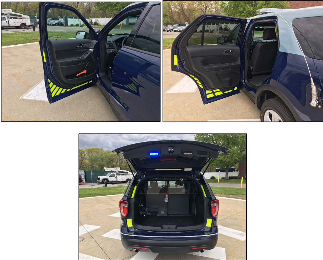
Figure 4: Retroreflective tape inside emergency vehicle doors and liftgate. Photo credit: Massachusetts State Police.
