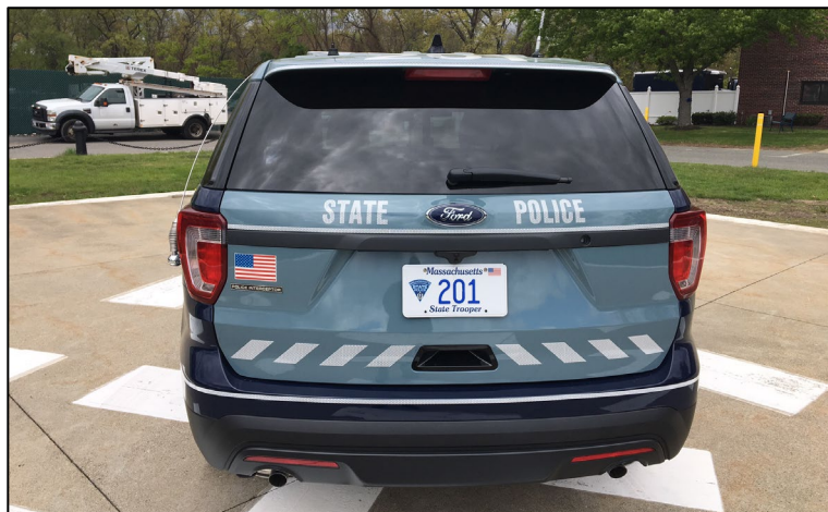
Figure 5: White retroreflective material in a chevron pattern on the rear of an MSP vehicle. Photo credit: Massachusetts State Police.
